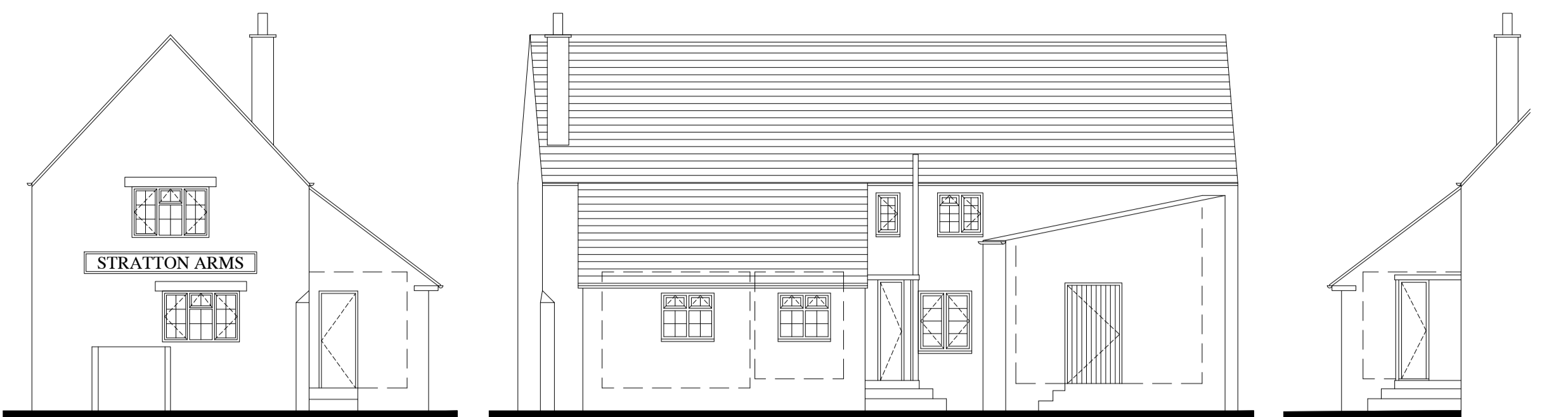
SIDE ELEVATION AS EXISTING REAR ELEVATION AS EXISTING SIDE ELEVATION AS EXISTING
