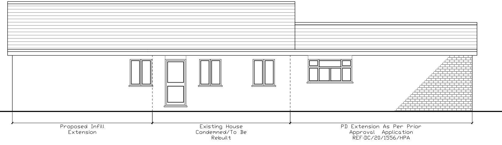
1:100 Proposed Side Elevation
