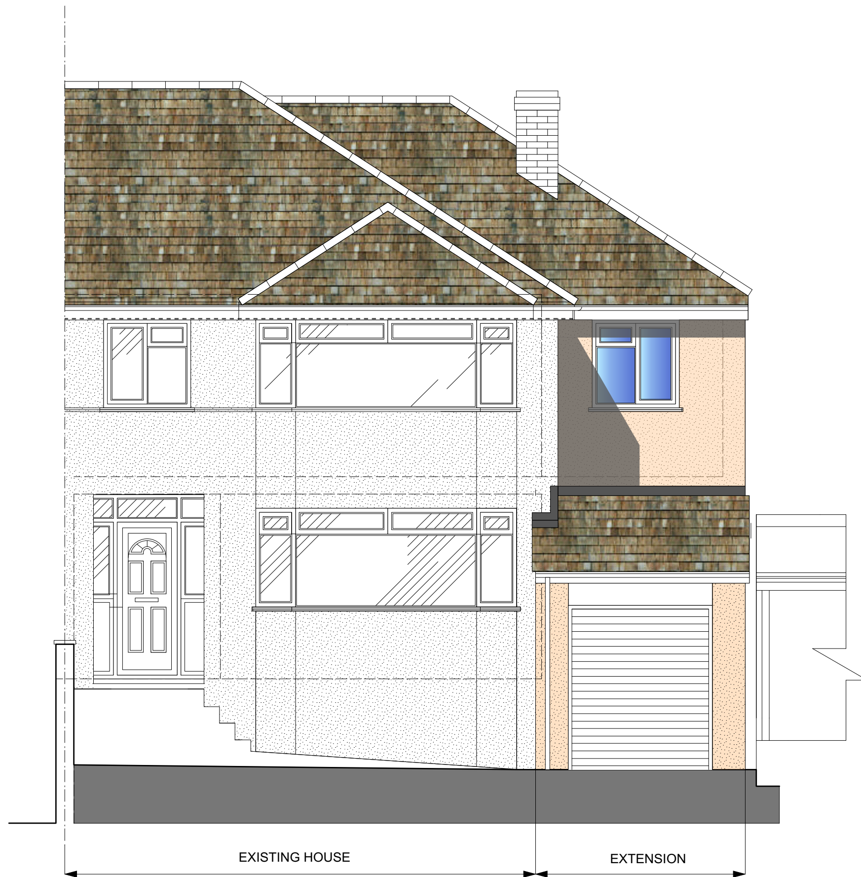
PROPOSED FRONT ELEVATION SCALE 1:50
