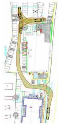
Image 7 – Swept path for a 12.6m urban artic delivery vehicle – not to scale
