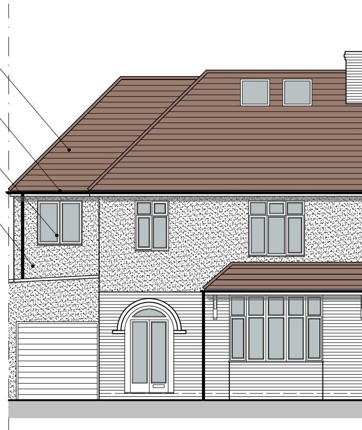
PROPOSED FRONT ELEVATION SCALE 1:100
