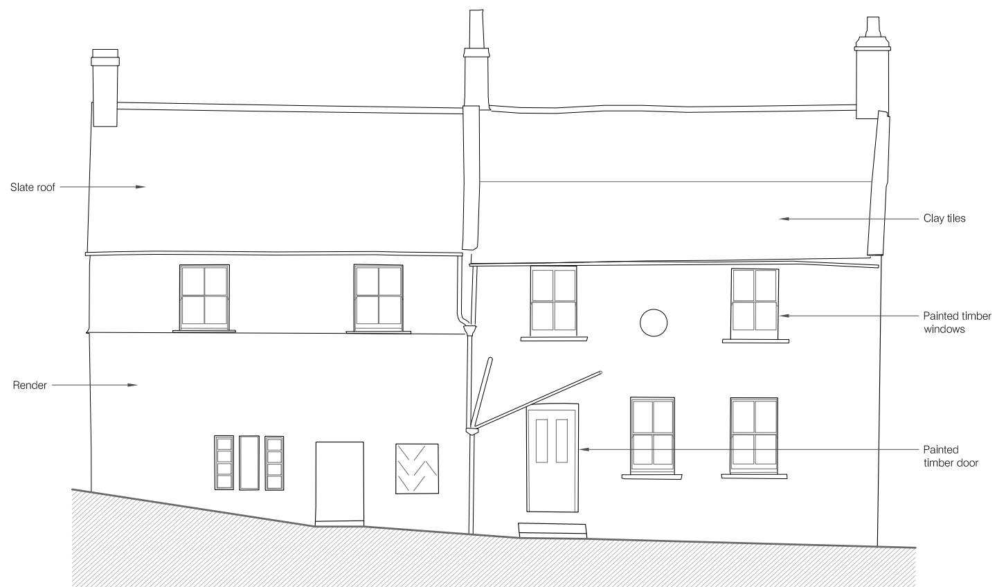
Existing South Elevation
