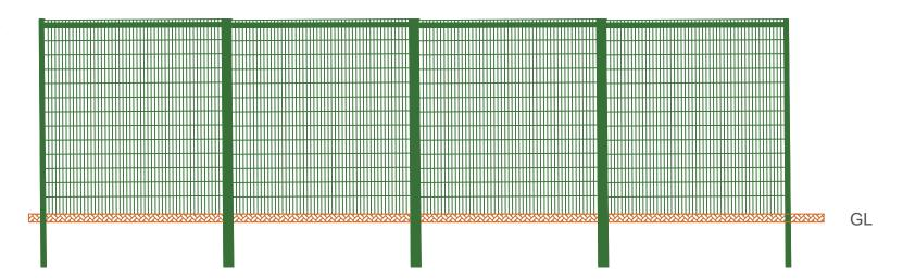
Proposed 2.4m Paladin Weldmesh Galvanised Steel Vision Panels in Green with Powder Coated Posts (1:50)
