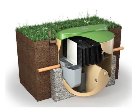
Fully compliant with EN12566-3 the Klargester BioTec domestic sewage treatment plant models are available in a variety of sizes 6-25 PE (UK) to suit any domestic application. The system employs the unique aerobic trickling process technology to filter and treat the sewage.
