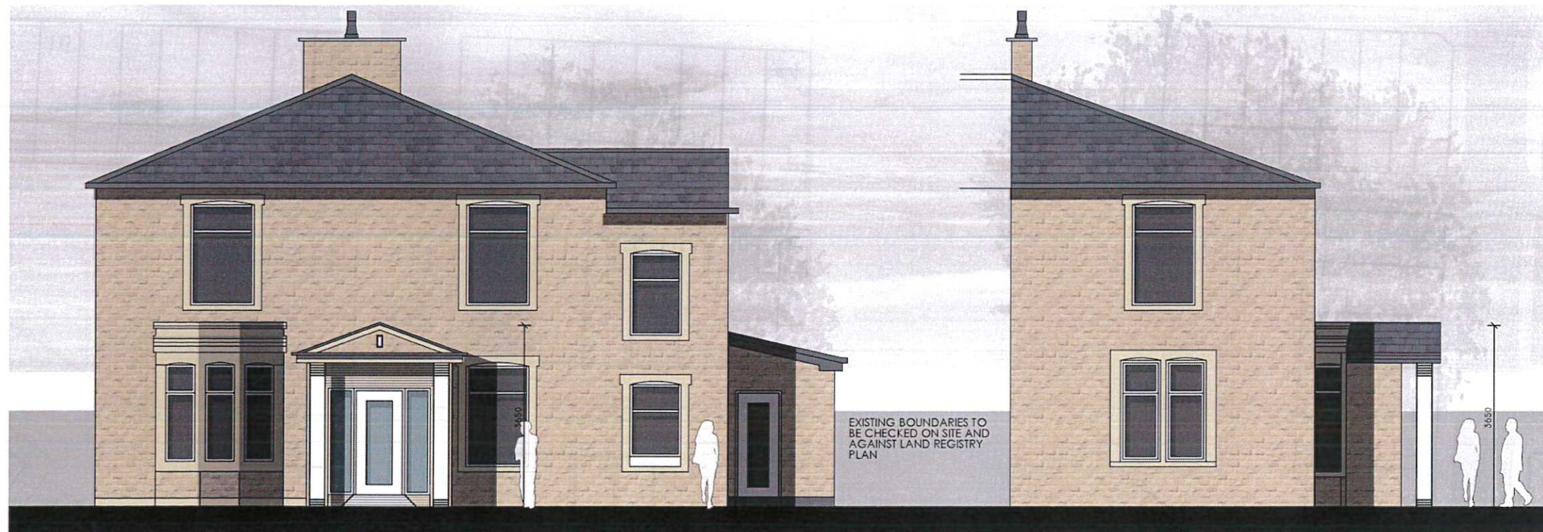
Proposed GF rear kitchen extension and front entrance porch with internal alterations and site works.
