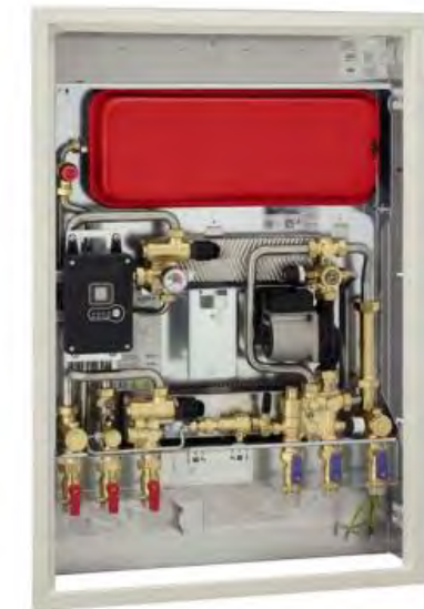
Figure 7.2.7 Caleffi SATK60103HE (590 H x 570 W x 110 D). Up to 28 kW DHW and 15 kW heating. This is a wall-mounted unit that can be recessed into the wall. This unit would only be able to meet the DHW demand of a studio apartment with a lowered DHW temperature of ~45°C.
