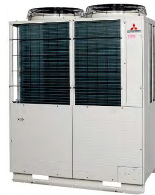
Figure 7.2.3 Example of an outdoor VRF heat pump unit, which can connect to several indoor units to provide simultaneous heating and cooling to different zones via a refrigerant branch controller box.
