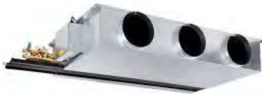
Figure 7.2.1 Example of a ceiling void-mounted horizontal fan coil unit. Warm air heating can be provided either by 4-pipe (chilled water and LTHW connections) or VRF variants.
