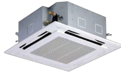
Figure 7.2.2 Example of a cassette-style indoor unit, mounted flush with the ceiling finish. Warm air heating can be provided either by 4-pipe (chilled water and LTHW connections) or VRF variants.
