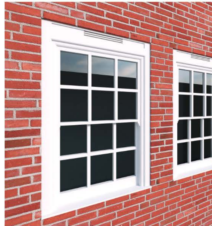
Rejected option - Incorporation of louvre into window frame
