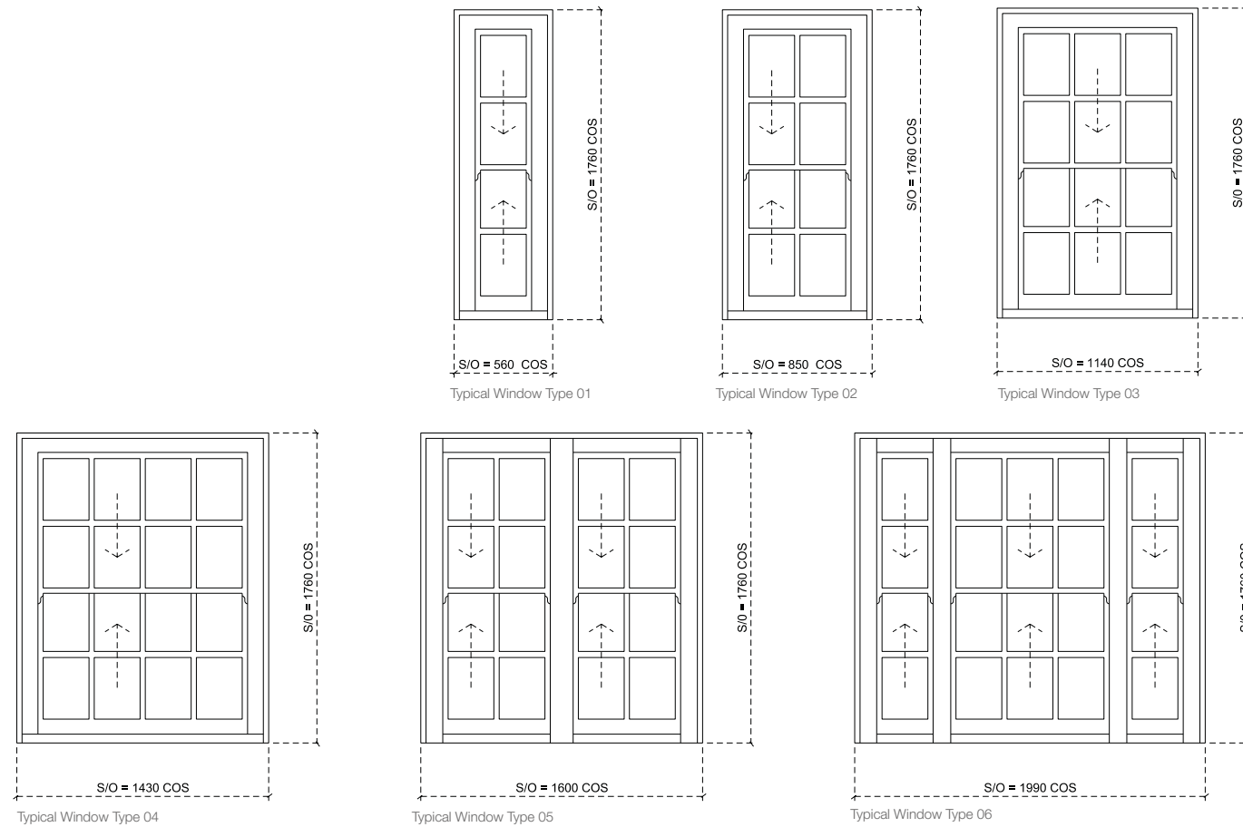
Fig. 4.3: Existing typical windows types and configurations
