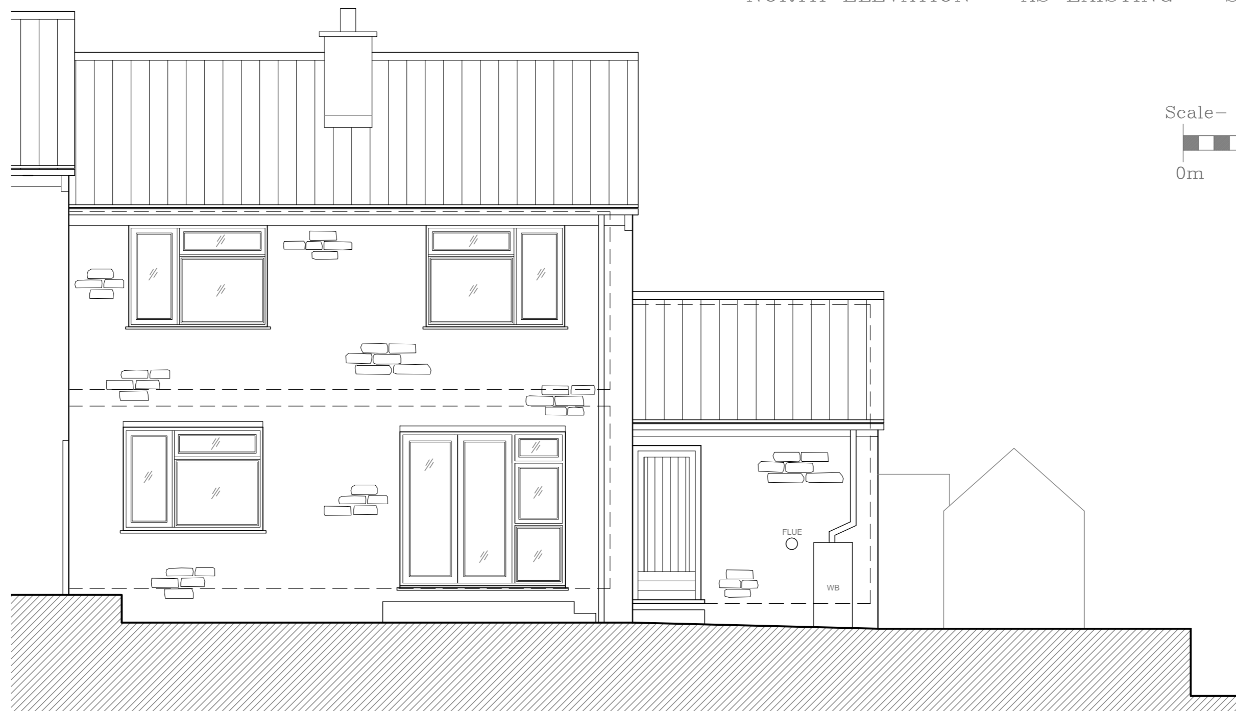
SOUTH ELEVATION - AS EXISTING - SCALE 1:50
