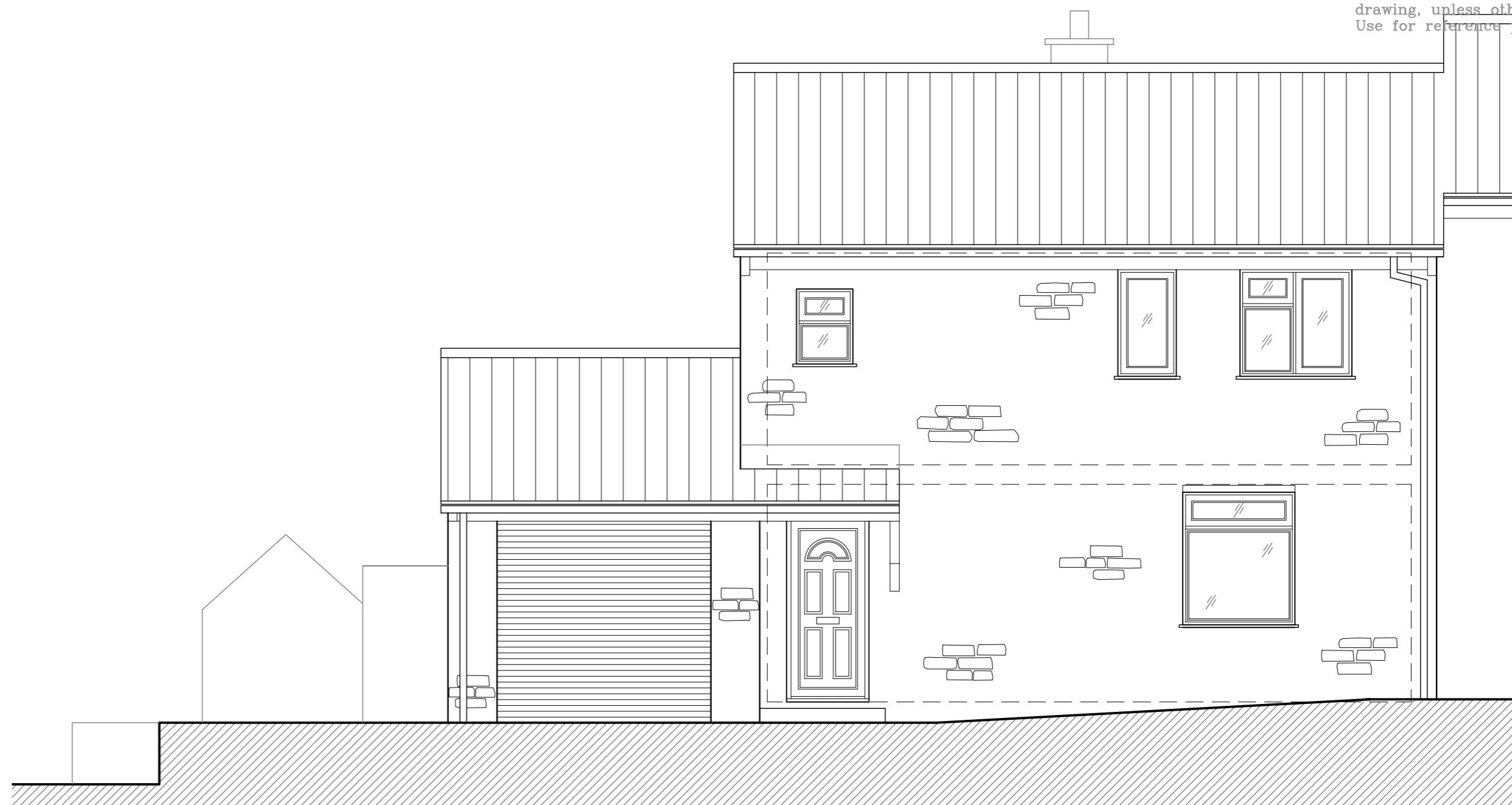
NORTH ELEVATION - AS EXISTING - SCALE 1:50
