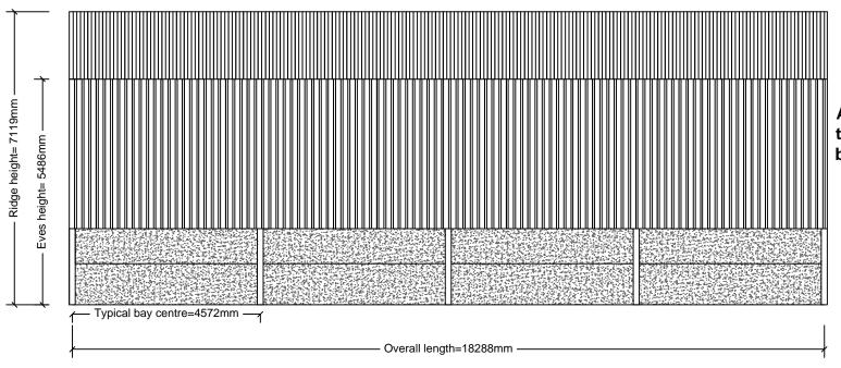
All vertical cladding to be treated timber boarding
