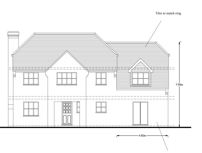
Front Elevation (North) Proposed wall construction to be face brickwork to ground floor and render to match extg on celcon standard blockwork to first floor, 100mm cavity fully filled with Drytherm insulation, inner leaf of standard celcon blockwork. Provide stainless steel cavity wall ties at 450cc vertically and 750mm cc horizontally. Double up ties each side of openings.
