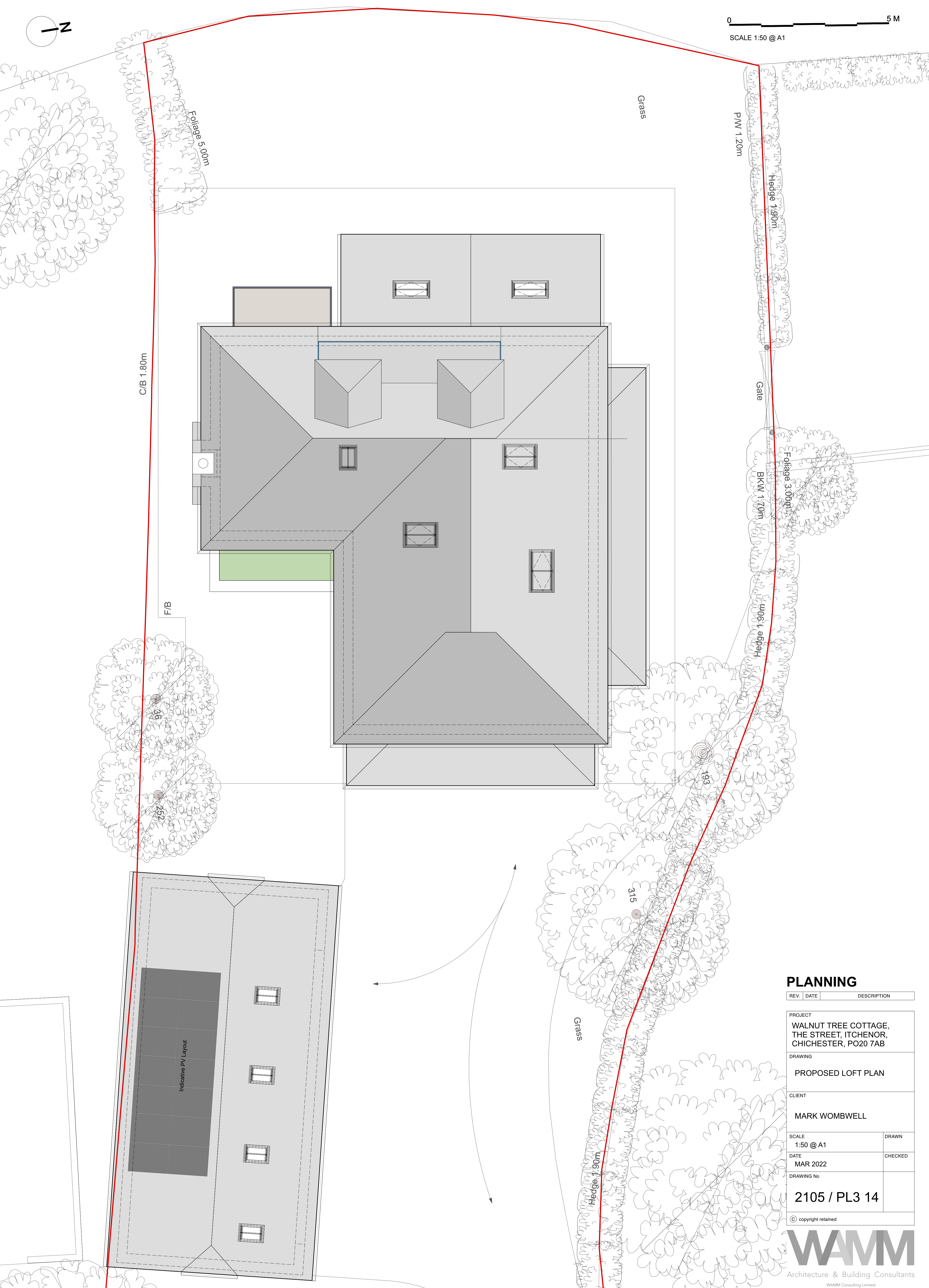
PROPOSED ROOF PLAN Scale: 1:50
