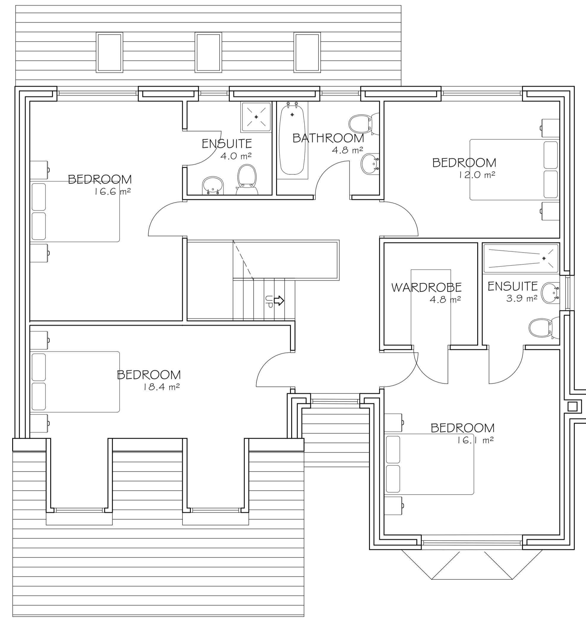
FIRST FLOOR LAYOUT TOTAL FLOOR AREA 96 m 2
