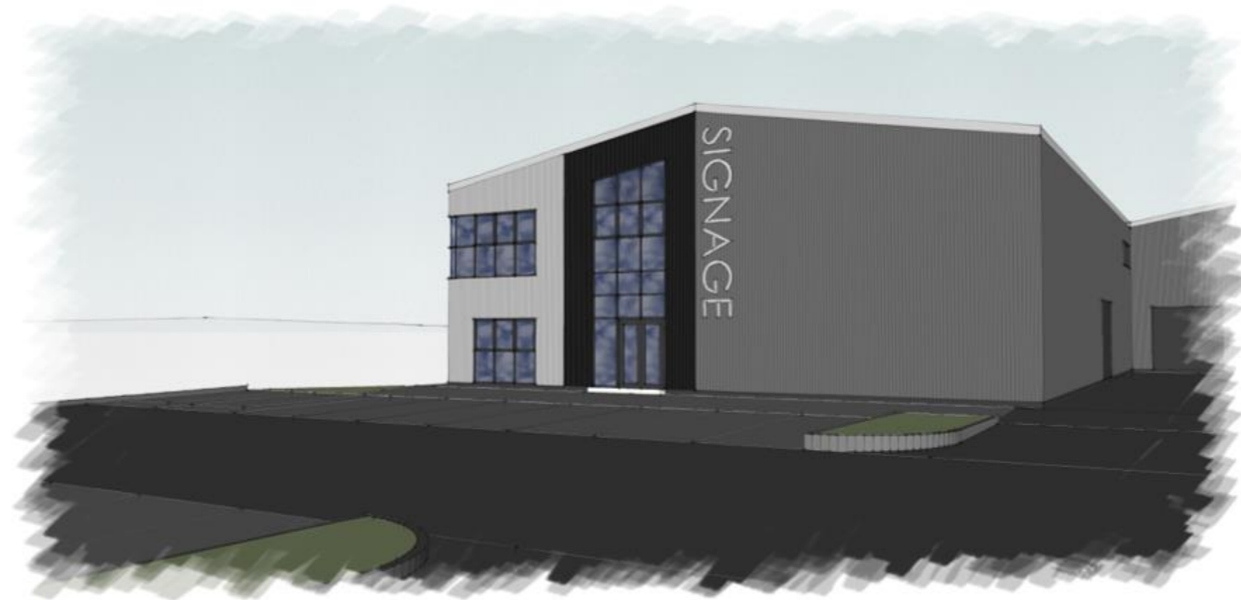
View from site entrance – double height curtain wall glazing feature at office entrance, changes in cladding break up the mass of the building
