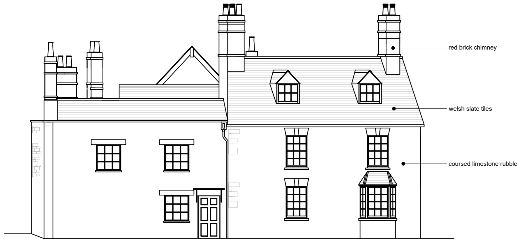
EXISTING ELEVATION 2 - EAST Scale 1:100
