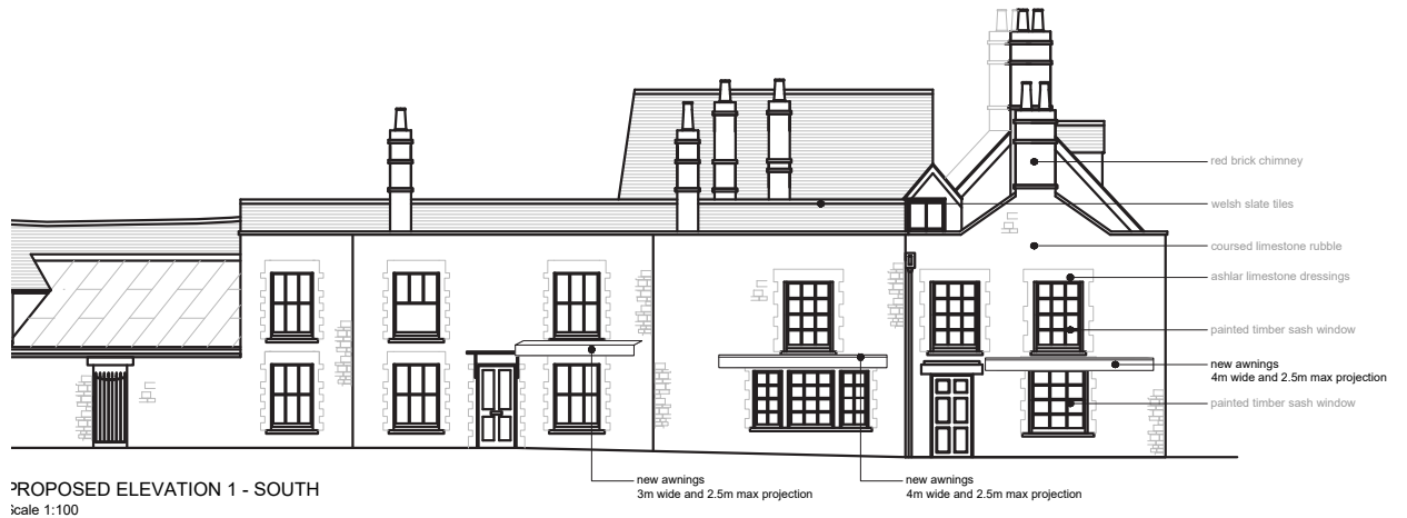
Fig.4.1 Proposed elevation with the awnings to the High Street elevation (not to scale).
