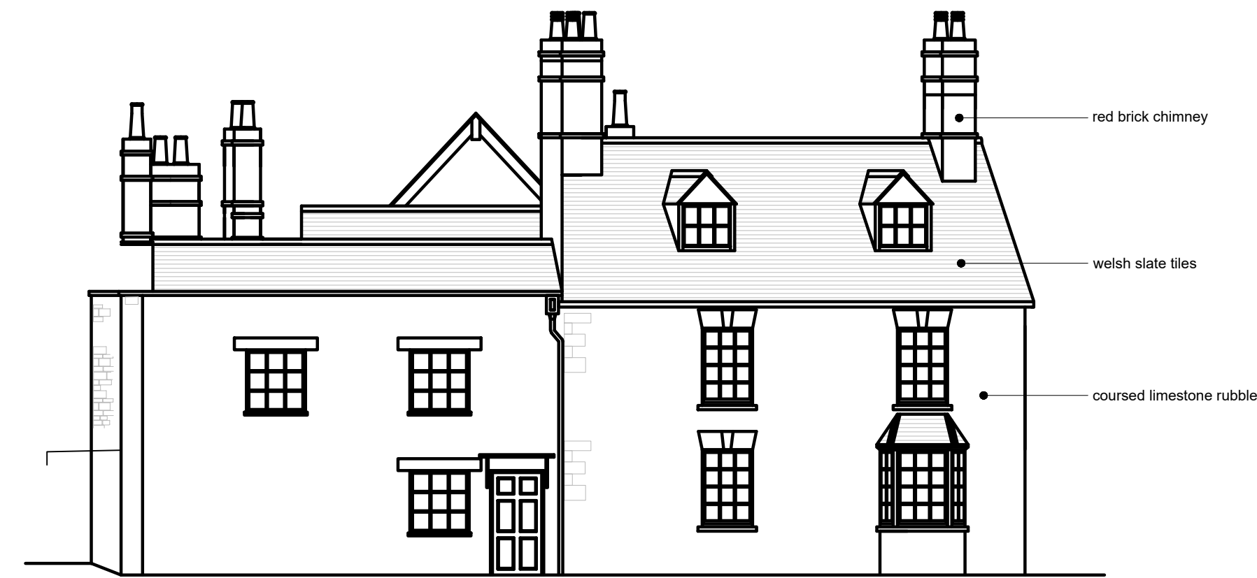
PROPOSED ELEVATION 2 - EAST Scale 1:100
