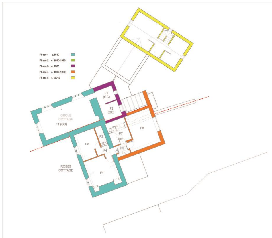
Fig.18 Sequential development of the first floors of Roses Cottage (lower) and adjoining Grove Cottage (upper)
