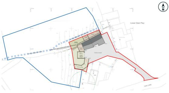
Proposed Site Plan – new access to field, relocate spring and subterranean garage
