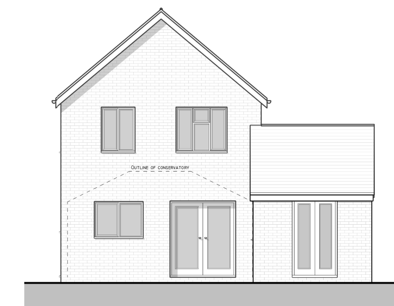
PROPOSED REAR ELEVATION 1 : 100
