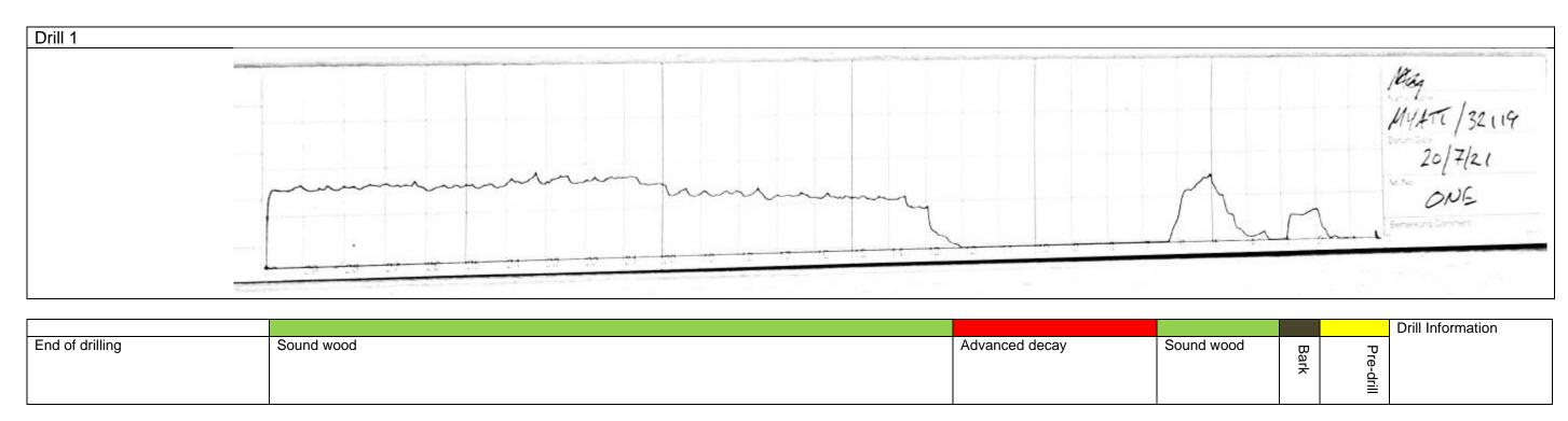
Notes and Discussion. This drill shows the bark with a small void beneath (delaminated from the sap wood), some sound but dead sapwood with an area of decay beneath, then going back into sound wood.
