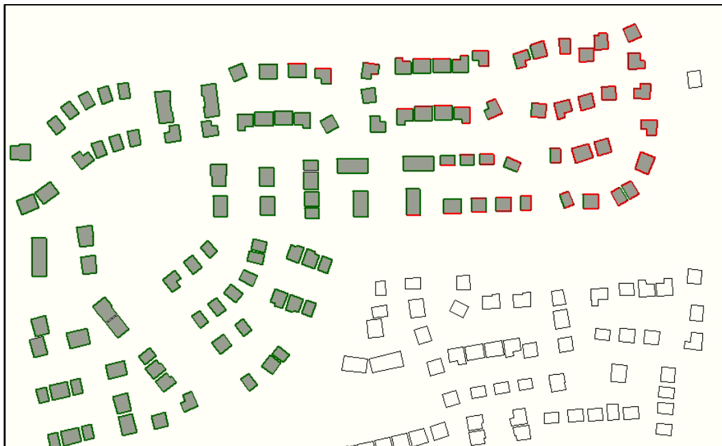
Figure 7 - Markup showing facades that require closed windows to achieve 'reasonable' internal criteria from BS8233 (Night 23:00-07:00)
