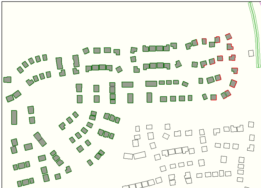
Figure 8 - Markup showing facades that require closed windows to achieve 'reasonable' internal criteria from BS8233 (Day 07:00-23:00) – with 2.5m bund along boundary
