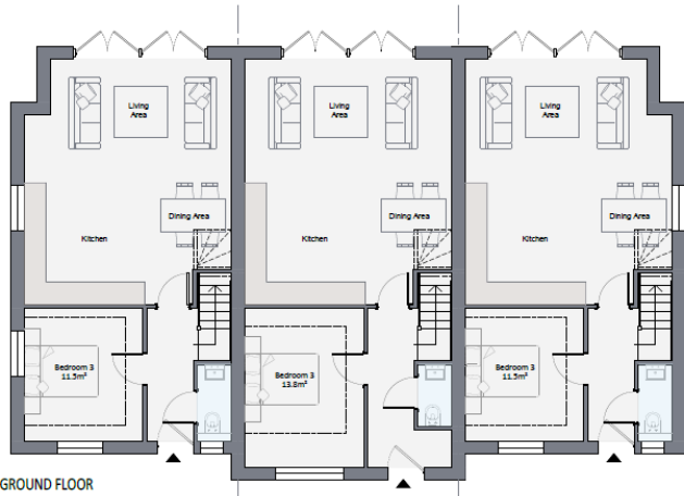
GROUND FLOOR PLOT 1- 107.0sq.m (1,152sq.ft) PLOT 2- 115.4sq.m (1,242sq.ft) PLOT 3- 107.0sq.m (1,152sq.ft)
