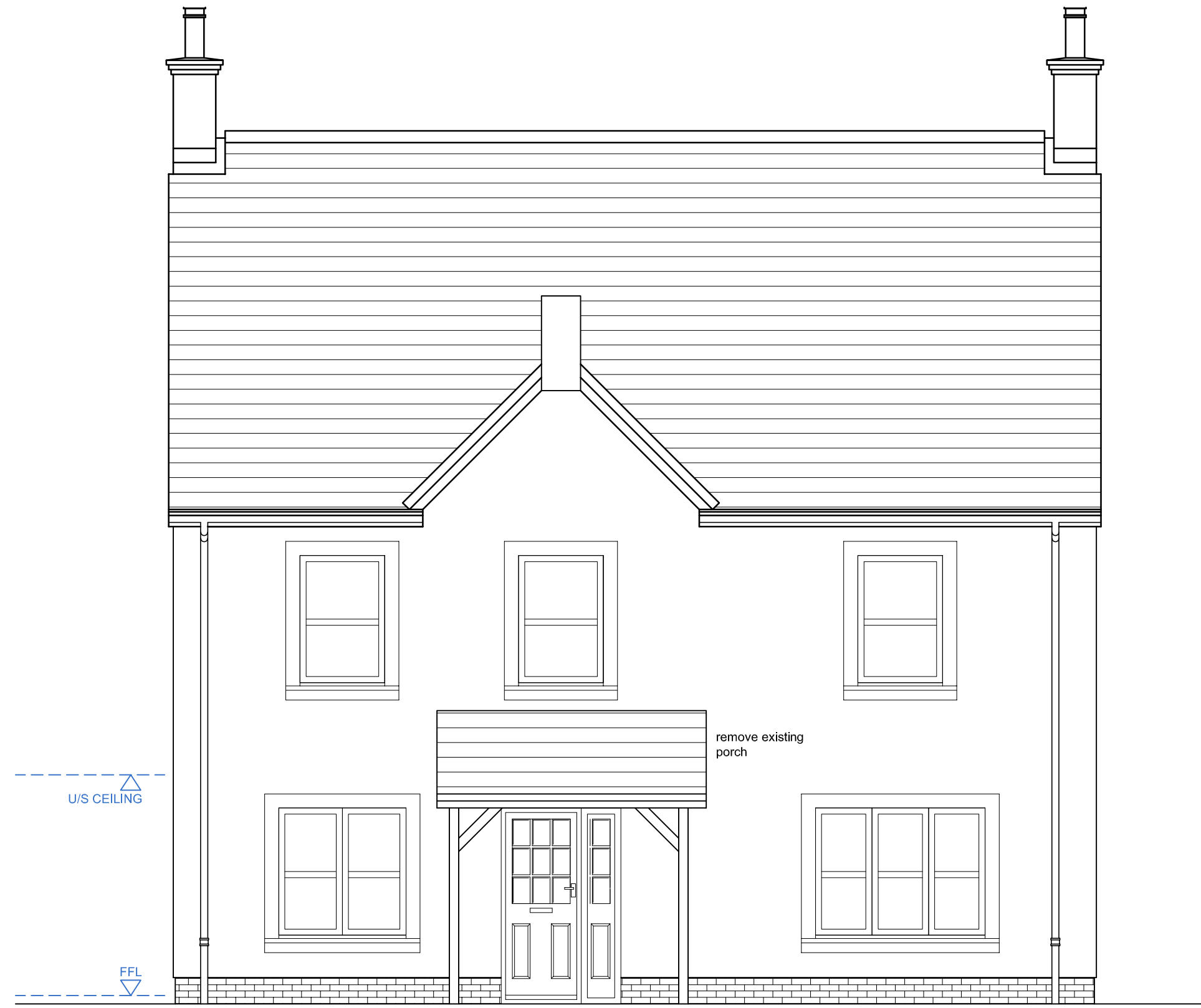
1:50 FRONT ELEVATION AS EXISTING
