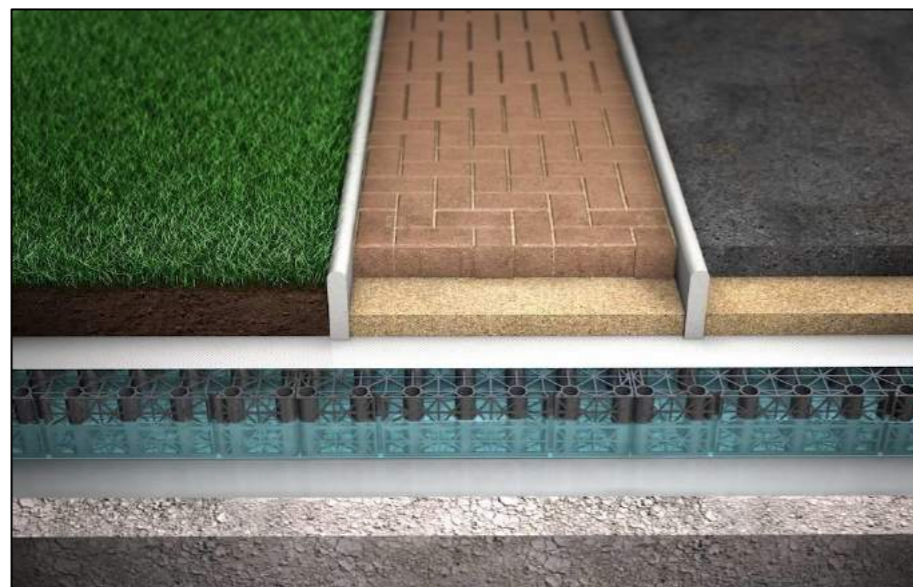
Figure 4-2 Permeable Paving with Geo-cellular sub-base
