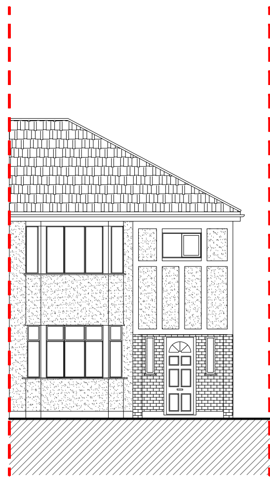
Existing Front Elevation
