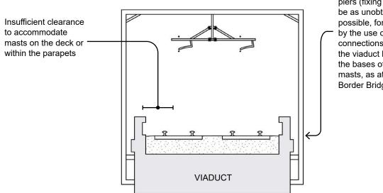
OLE mast fixed to the elevation, over the piers (fixing detail to be as unobtrusive as possible, for example, by the use of structural connections through the viaduct between the bases of the masts, as at the Royal Border Bridge, below)
