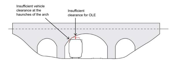
Typical constraints for the installation of OLE wires under an existing bridge
