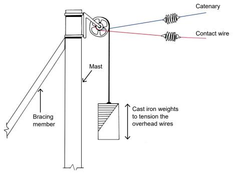
Cast-iron balance weights, as traditionally used on UK railways (a 'balance weight anchor')
