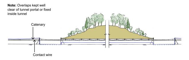
**Running OLE wires through tunnels**
