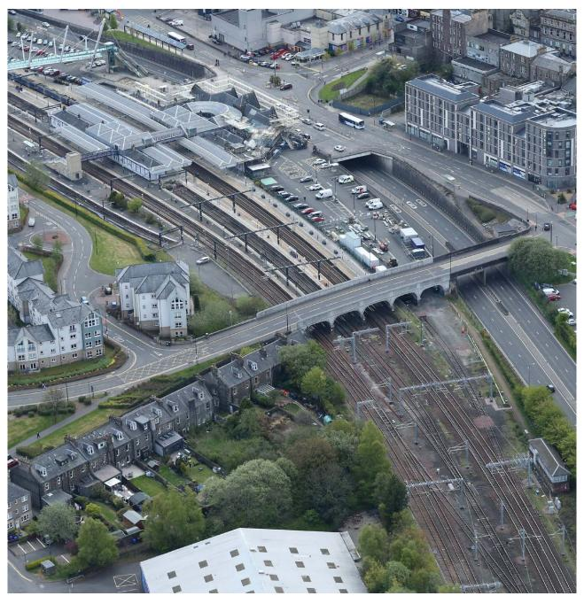
Stirling Station from the air, showing how the OLE on the platforms has been carefully ordered to create a harmonious visual effect, in contrast to the OLE on the other side of the road bridge (photograph: © Network Rail)
