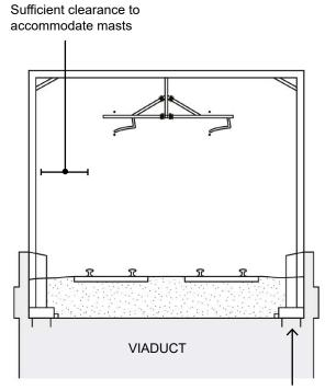
OLE masts supported on viaduct deck within the width of the parapet if there is sufficient clearance between the track and the inner edge of the parapet
