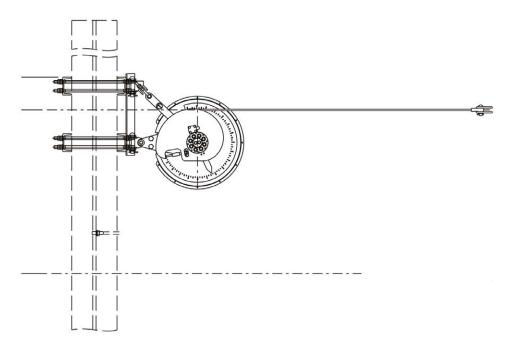
Spring tension device 'tensorex', as now used on electrification projects
