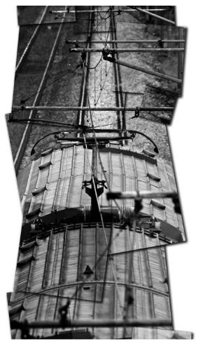
Stagger of contact wire and catenary. Note also the pantograph on top of the train (photograph ©Graeme Bickerdike/Four by Three)
