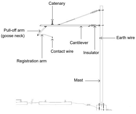
An example of an OLE mast, cantilever and associated equipment (in this case, 'UK Master Series')
