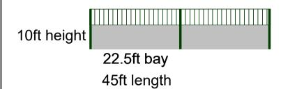
West elevation will have a 6ft high concrete blockwork with juniper green box profile sheeting above and on the roof.
