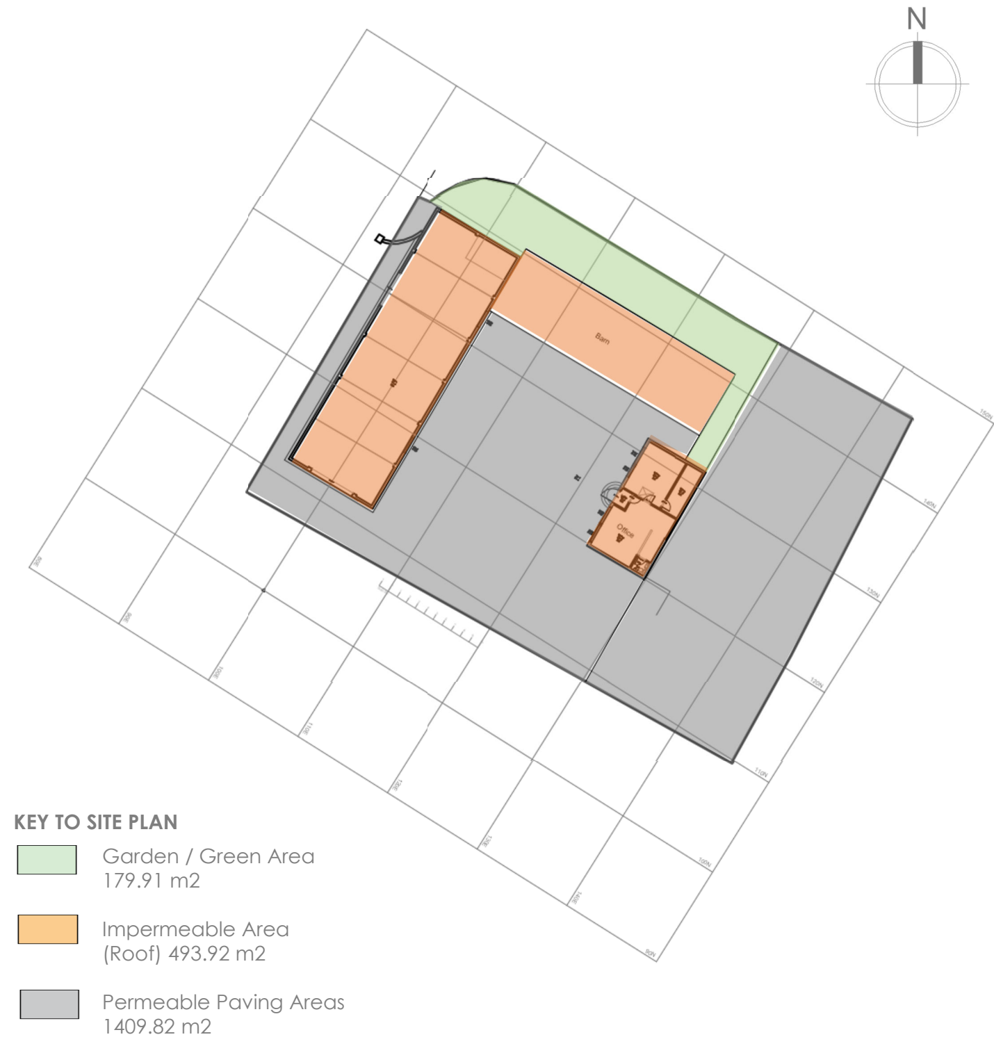
FIGURE 7 –GROUND FLOOR SITE PLAN AS EXISTING
