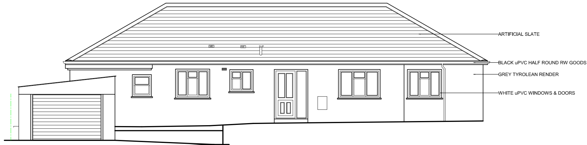
EXISTING NORTH ELEVATION (FRONT)
