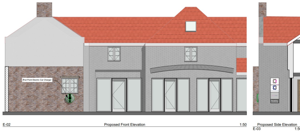
Elevations with the Car charger
