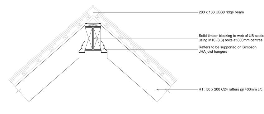
Beam & Plate Detail scale 1:10
