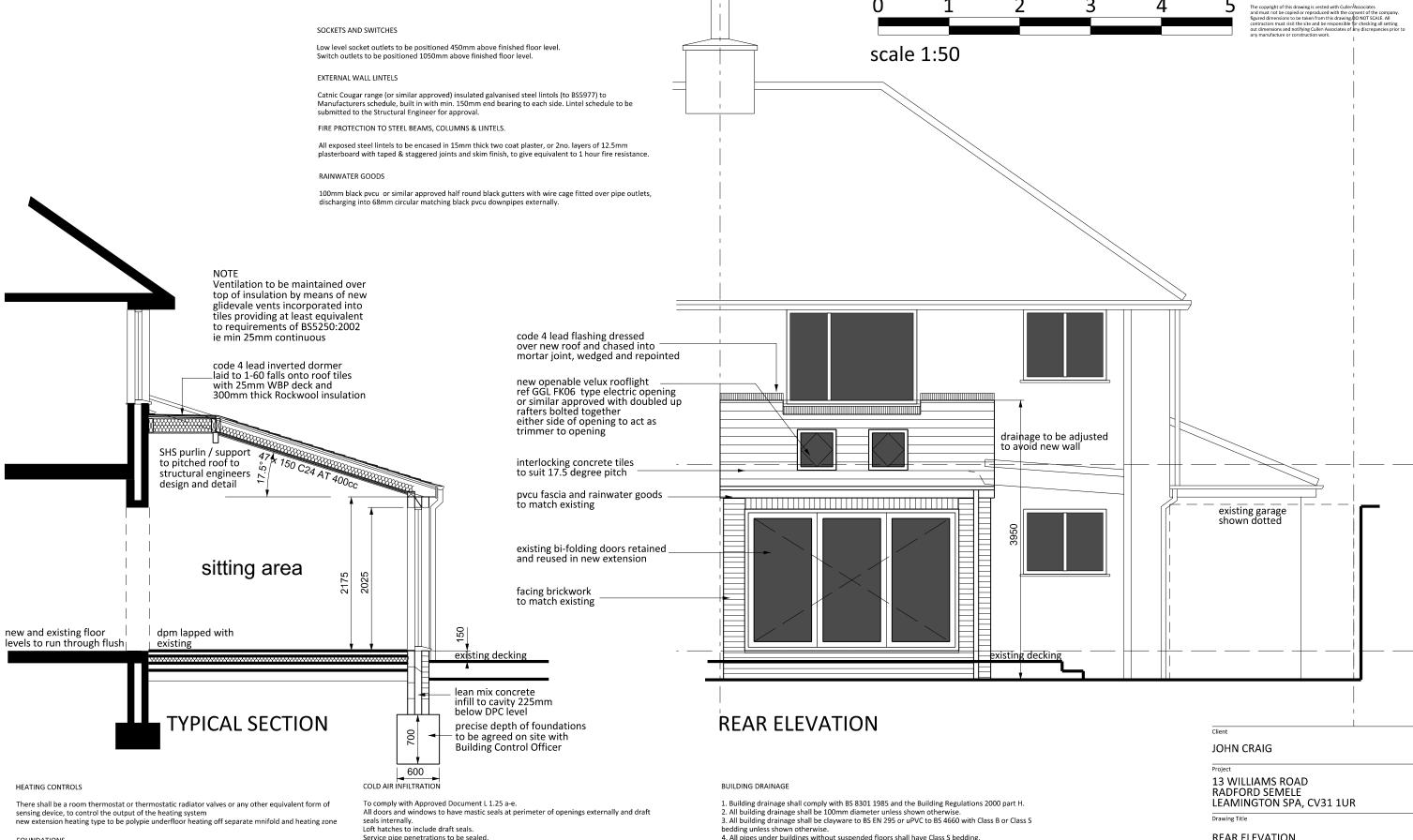
600mm wide concrete trench fill foundations at a depth to be agreed on site with local authority building control officer. If on site inspection ground conditions dictate special foundations. Structural Engineer to be appointed to design & detail foundations. Min mix of concrete to be ST1, in strict accordance with BS5928 1981, foundation trenches to be
