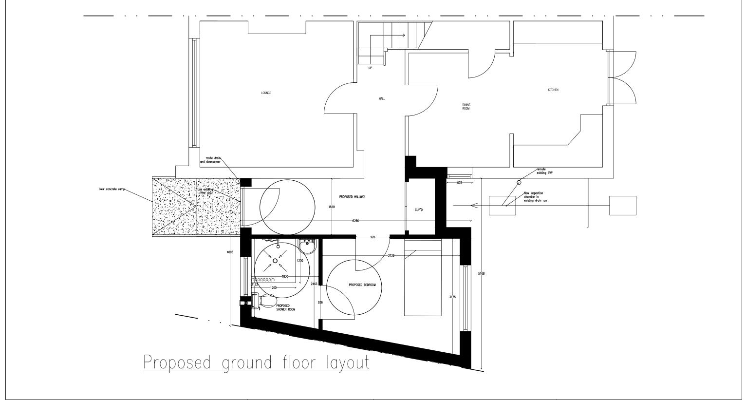
All dimensions to be checked on site prior to commencement of work. Do not scale from the drawing, use figured dimensions only.
