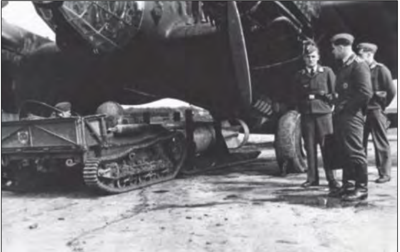
Above: A Heinkel He 111 P-4 (same variant as that which crashed near the site) in Chartres, France in April or May 1941 with a 500kg bomb being loaded by a captured French light carrier.
