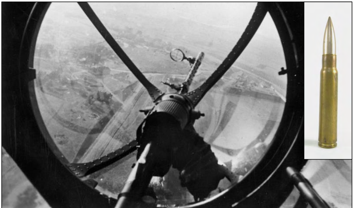
Below: An MG-15 shown mounted in a Heinkel He 111 over Poland in 1939. Next to it is the 7.92x57mm Mauser small-arms ammunition that it fired. These machine guns were the most common kind mounted on the He 111.
