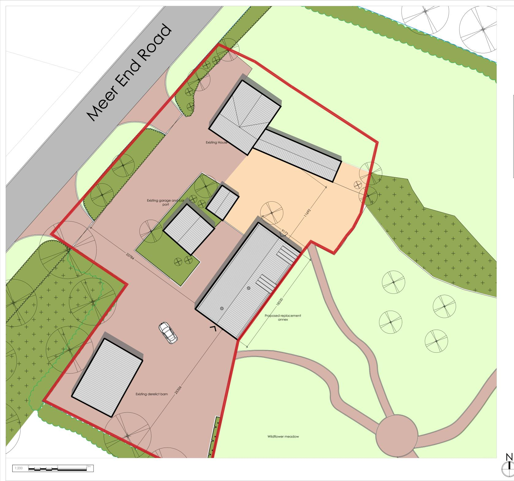
Site layout legend: Proposed site boundary Gravel area Proposed tree planting Tarmac finish Existing tree planting (root protection in red) Block paving X Areas laid to Removed trees grass Surger a - 1.8m close boarded timber fence 1.8 CBF Low level landscape planting
