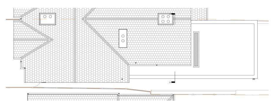
**PROPOSED ROOF PLAN** Scale 1:100
