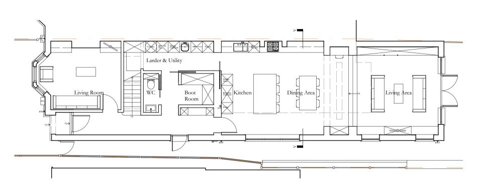
**PROPOSED GROUND FLOOR PLAN** Scale 1:100
