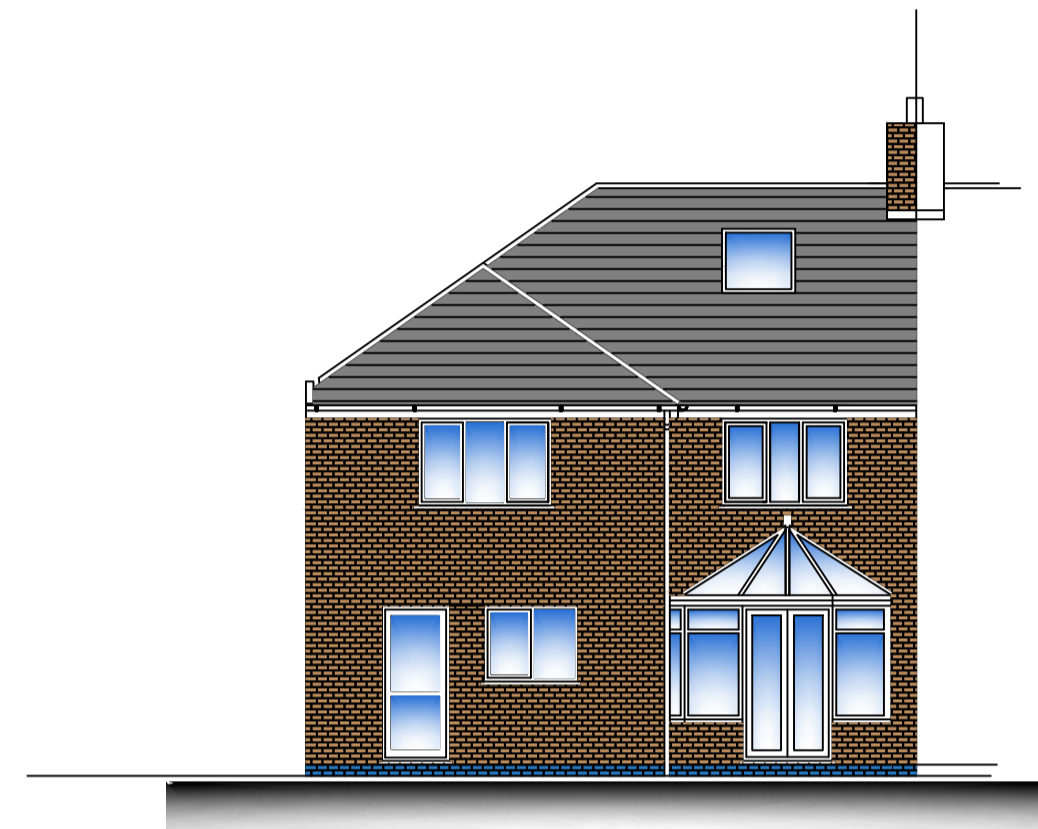
EXISTING REAR ELEVATION
