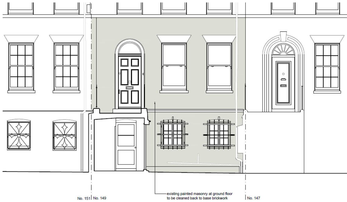
Figure 7: Existing front elevation
