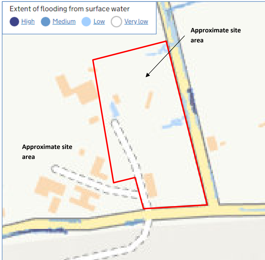
Figure 7.1 – Surface water flooding extents
