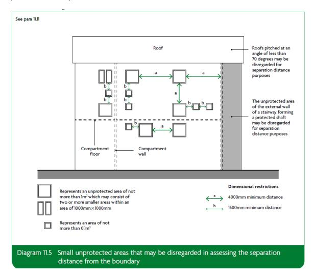
The diagram is copied below. It is possible to have permitted unprotected openings closer to each other than shown by the green lines in the diagram, where the relevant windows are in different apartments, because the assumption is that a fire would not spread between apartments.
