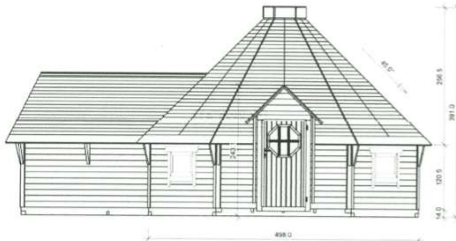
Front elevation of glamping pod
