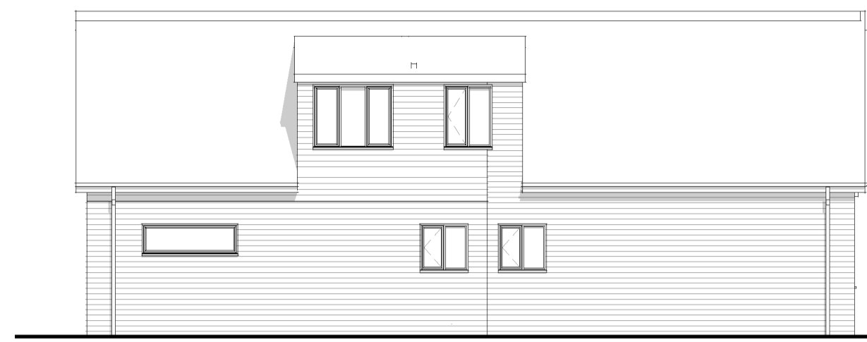
Garage - East Elevation 1:100
