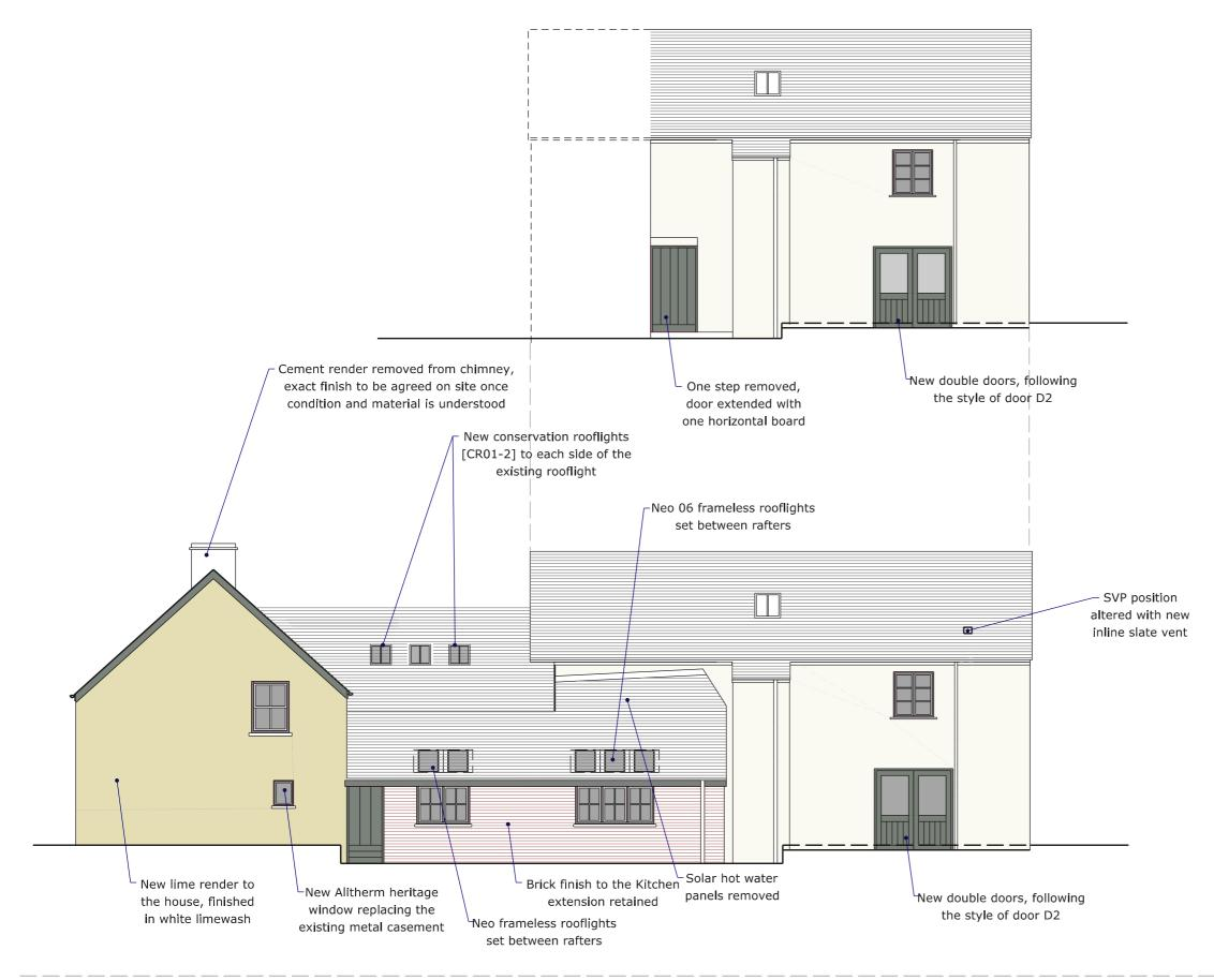
Revisions: A - Additional information added Lamb House, Glasbury South Elevation - As Proposed 1001.08A 1:100@A3
