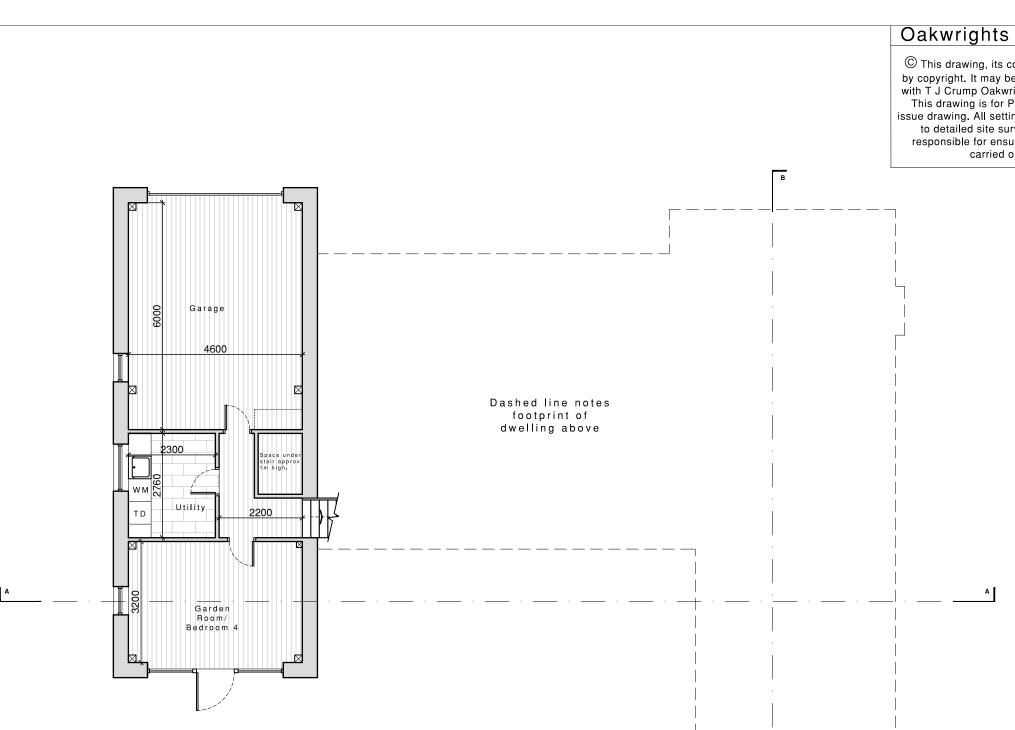
PROPOSED BASEMENT FLOOR PLAN SCALE 1/100
